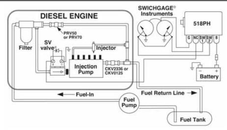
**NOTE:** Mount the SV valve as close as possible to the injection pump. If using the SV valve with electronic devices, we recommend installing a suppression diode across the SV valve coil.
